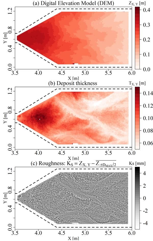
Figure 6: Bed topography data: a) Bed elevation  $Z_{X,Y}$ ; b) Deposit thickness  $T_{X,Y}$ ; and c) Surface roughness  $Ks_{X,Y}$  (GSD2,  $Ql=2.2$  l/s,  $t=25$  min)
